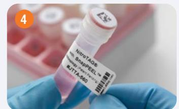
4 Apply the rectangle to the side of the cryo vial
